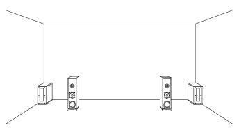
Dual corner placement provides maximum output from each sub, higher total output, good "imaging" and more even room response.
